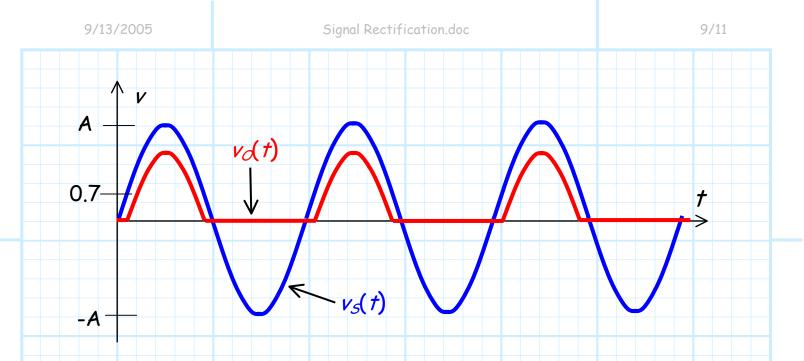
Although the output is **shifted downward** by 0.7 V (note in the plot above this is **exaggerated**, typically  $A \gg 0.7$ V), it should be apparent that the **output** signal  $v_{c}(t)$ , unlike the input signal  $v_{s}(t)$ , has a **non-zero** (positive) **DC component**.
