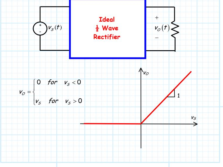
Pretty simple! When the input is negative, the output is zero, whereas when the input is positive, the output is the same as the input.
