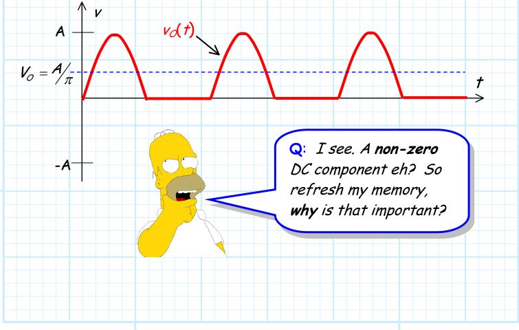
A: Recall that the **power distribution** system we use is an AC system. The source voltage  $v_{s}(t)$  that we get when we plug our "**power cord**" into the wall socket is a 60 Hz **sinewave**—a source with a **zero DC component**!
